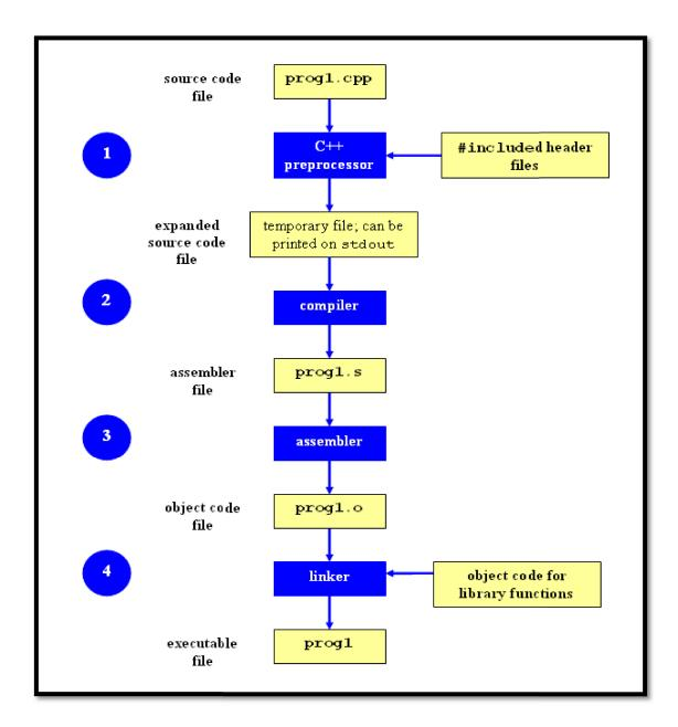
Compiling a source code file in C++ is a four-step process. For example, if you have a C++ source code file named prog1.cpp the compilation process looks like this:
